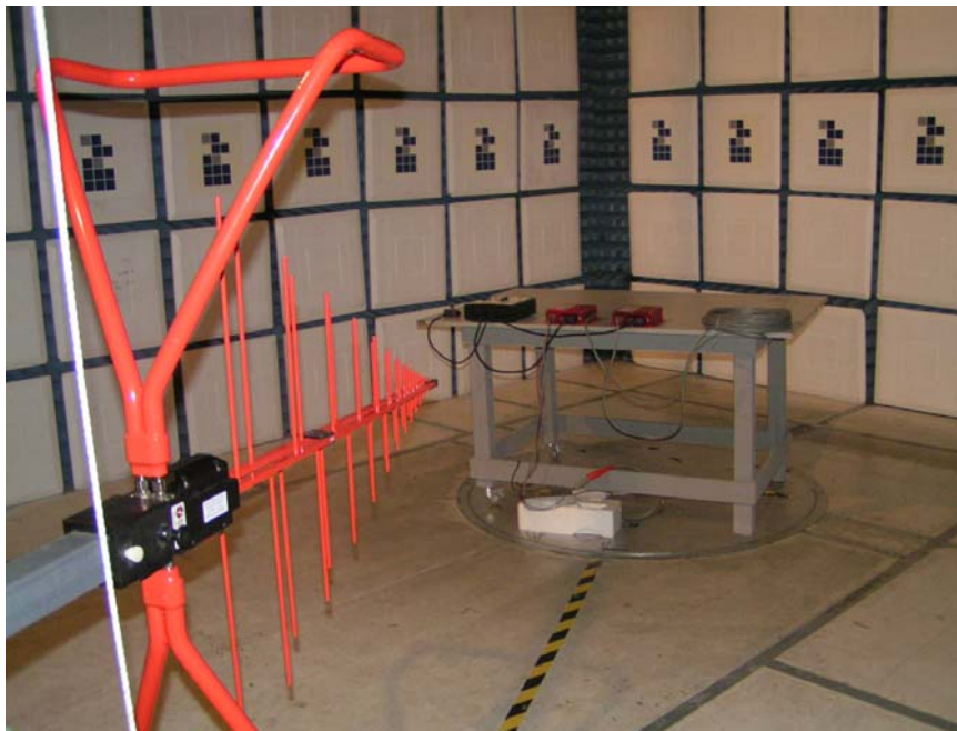
Radiated Emission Test Set-up Back View
