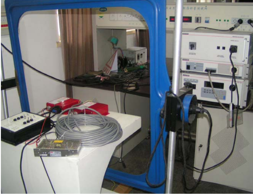
Power Frequency Magnetic Field Test Set-up
