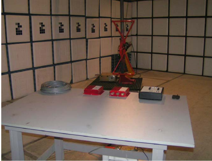
Radiated Emission Test Set-up Front View
