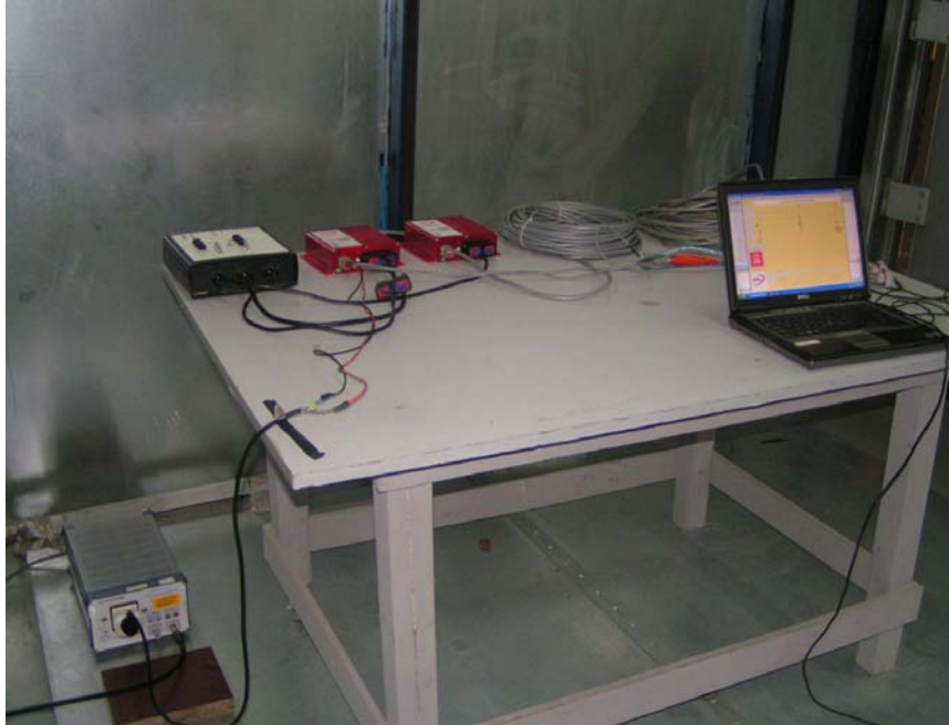
Conducted Emission Test Set-up Front View
