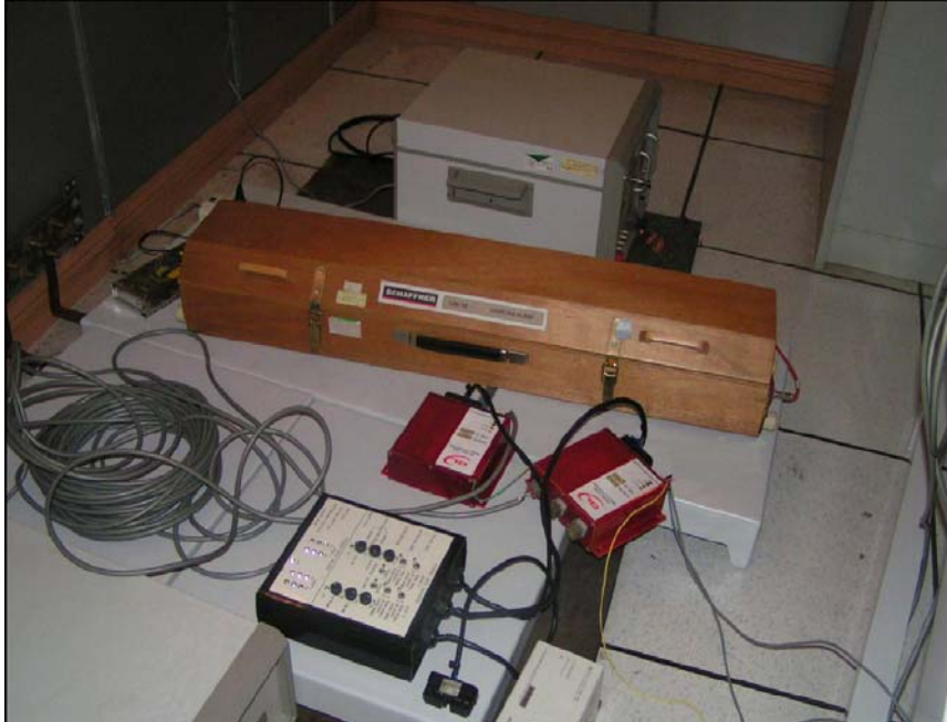
Conducted Immunity Test Set-up
