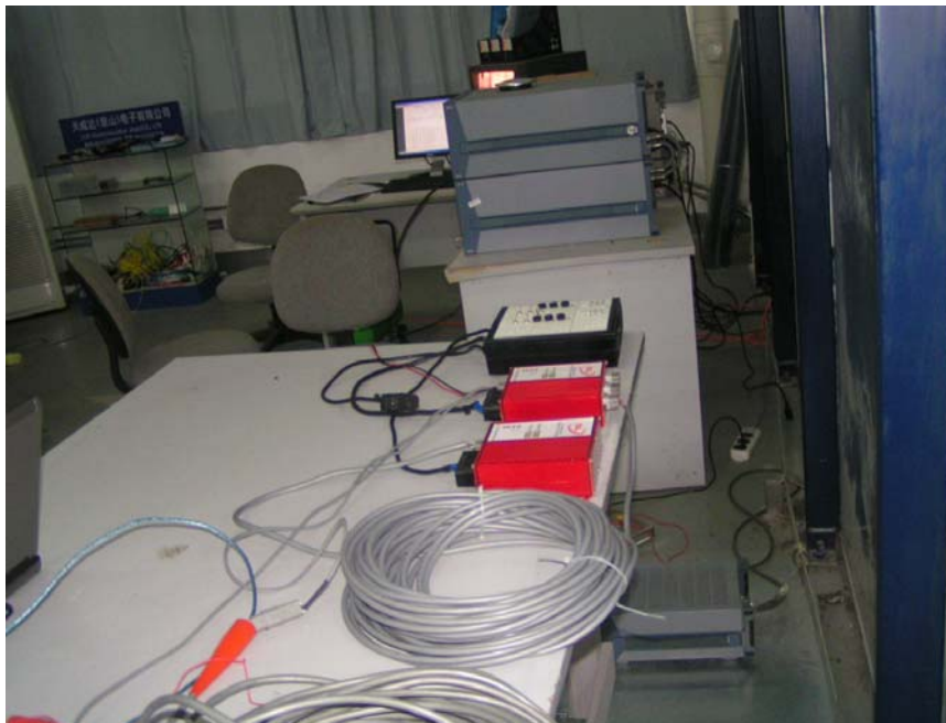
Conducted Emission Test Set-up Side View
