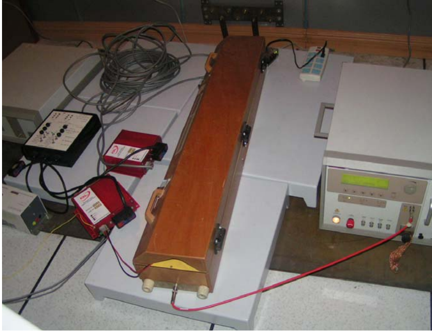
Electrical Fast Transient/Burst Test Set-up
