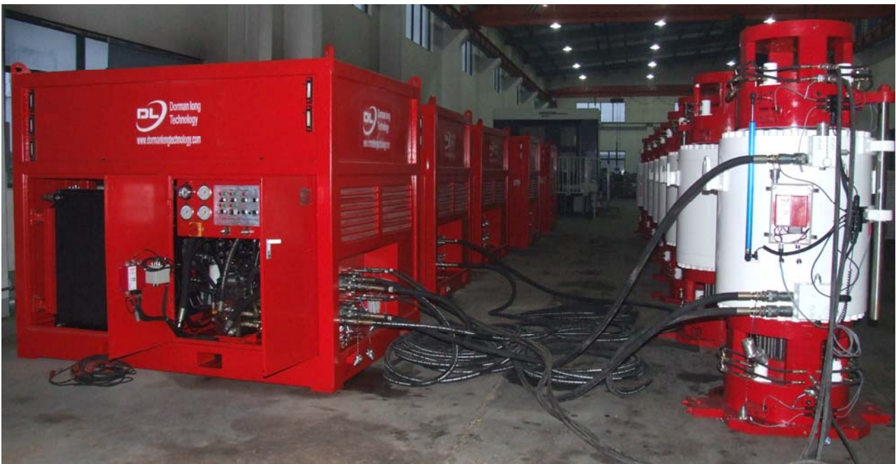
DL-L120F/2/300/D diesel powered hydraulic power packs during pressure and function testing
