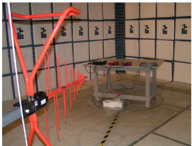
Radiated Emission Test Set-up Back View
