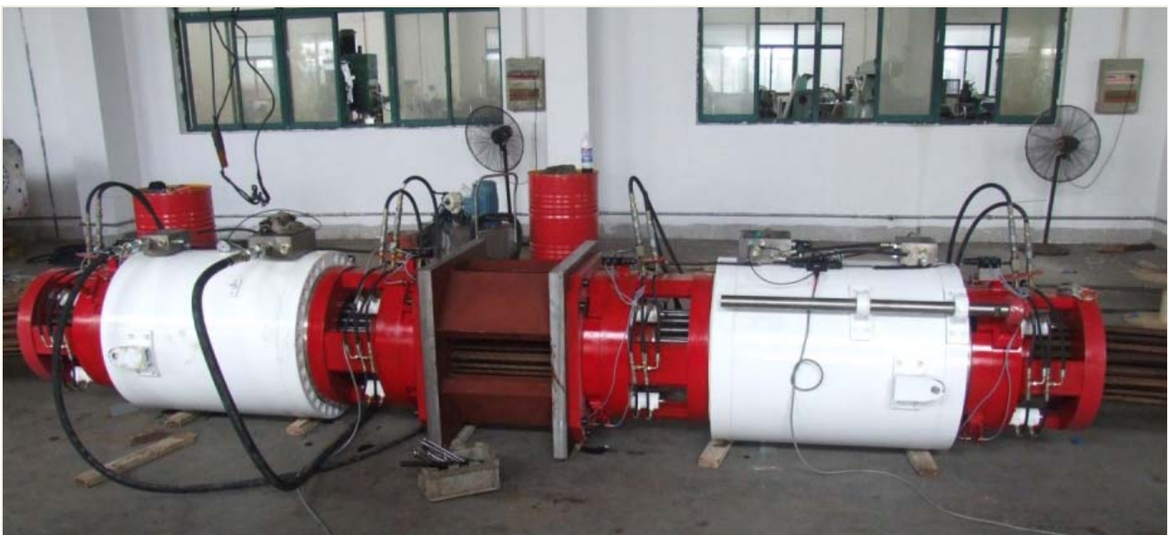
DL-S588 strand jacks undergoing back to back 125% load test prior to delivery
